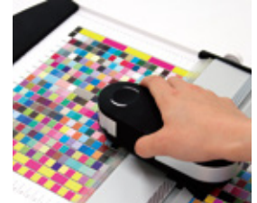
Color measurement with a colorimeter
